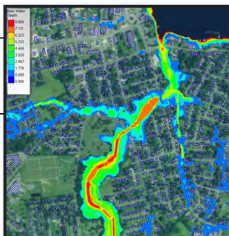
With protective berms – maximum water depth, 25-year storm event (right)
